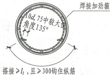
搭接  $\geq l_1$ , 且  $\geq 300$  钩住纵筋
