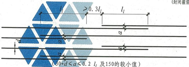
**非接触纵向钢筋搭接构造**
